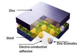
As a consequence of the unique manufacturing process and the high pureness of the employed zinc, the band has an absolutely homogeneous and isotropic microstructure, which cannot be found in other protection systems. For this reason, any pitting or any form of local corrosive attacks are avoided. Therefore we can state that, owing to the following features:
