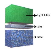
the two surfaces are no longer connected in the right way. This will not happen when employing our zinc tape with electro-conductive adhesive. Through our zinc coating on the iron surface passive and active protections can be achieved:
